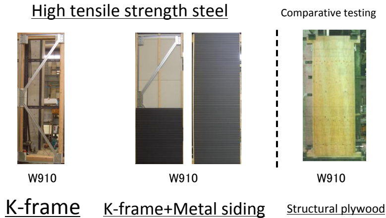
Fig.18. Specimens model (retrofitting equipment with high-tensile steel)
