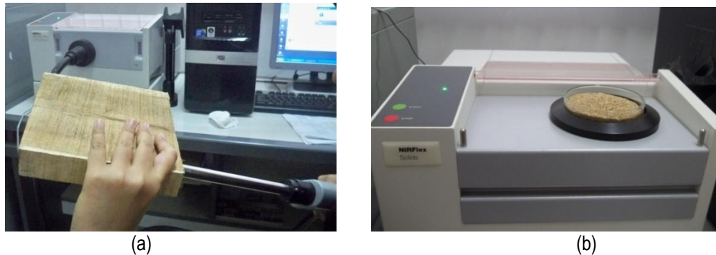
Gambar 1. NIR spectroscopy testing using NIRFlex N-500 fiber optic; solid wood sample, (b). ground wood sample
