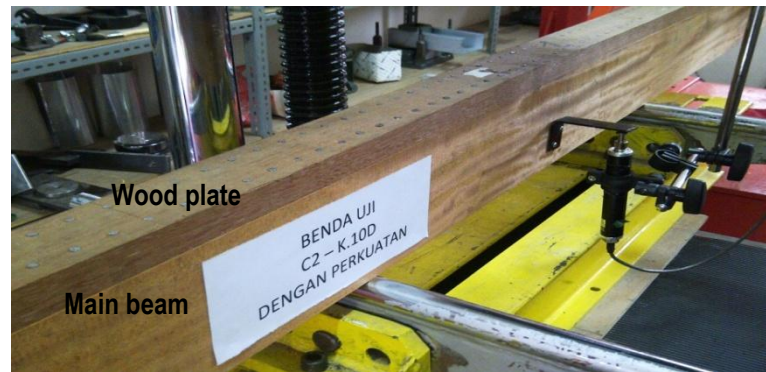
Figure 3. Two rows with 10d (20 mm) spacing of nails at MK-10D-2 specimens.
