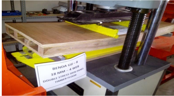
Figure 8. Setting of the specimen on the third point loading test
