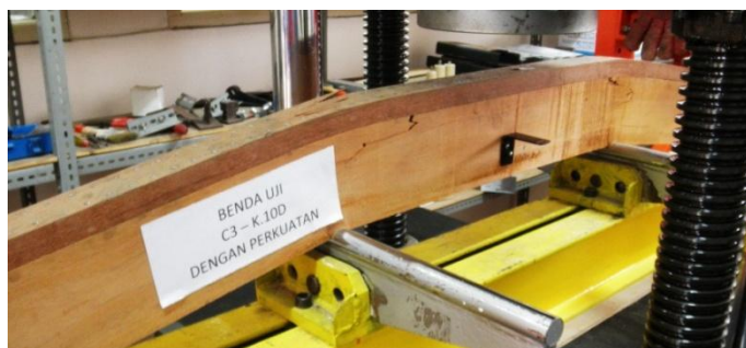
Figure 13. Tension failure on the main beam MK-10D-2
