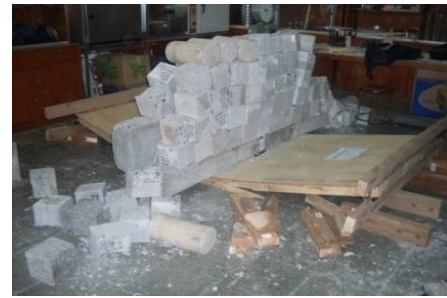
Figure 2b. Specimen at failure at 15 kN line loading
