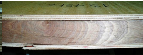
Figure 13b. Tension failure at plywood
