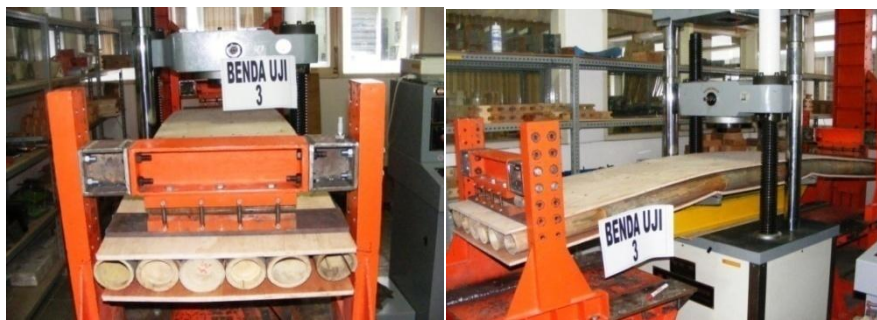
Figure 3. The Composite plywood-bamboo floor specimen under loading test
