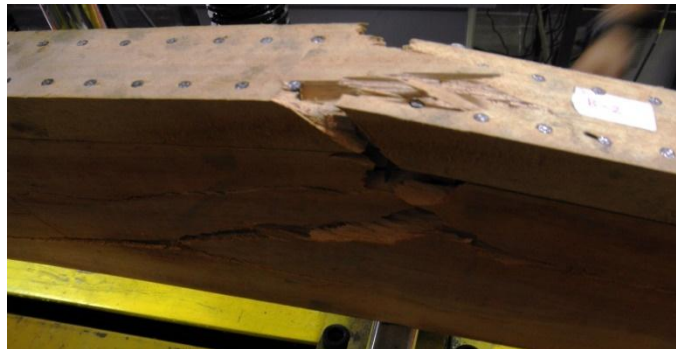
Figure 12. Tension failure at wood plate following by tension failure on the main beam MM-10D-2
