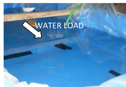
Figure 1b. 500 mm height of water as a uniform loading, without failed.
