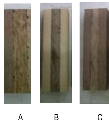
A = OPT/ compressed-OPT/ OPT B = Sengon/ compressed-OPT/ Sengon C = Meranti/ compressed-OPT/ Meranti
