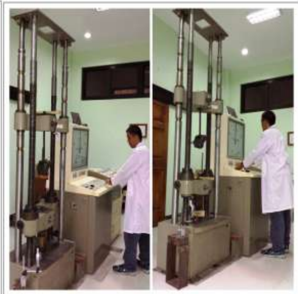
Appendix 10. Compression parallel and perpendicular to grain test.
