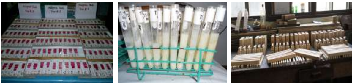
Appendix 6. Specimens/wood samples prepared for a) wood anatomical observations and descriptions; b) fiber and vessel mensurations; and c) strength and related properties determination.
