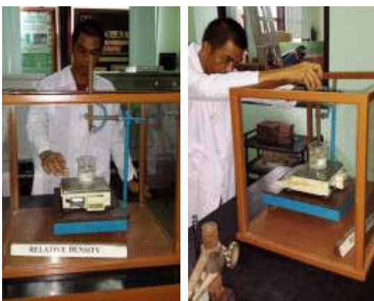
Appendix 7. Weighing of wood sample for moisture Content and relative density determination
