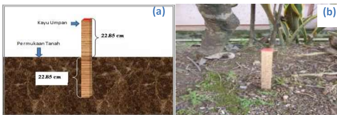
Figure 1. Assembled stake, (a) Sketch of assembled stake, (b) Assembled stake in location
