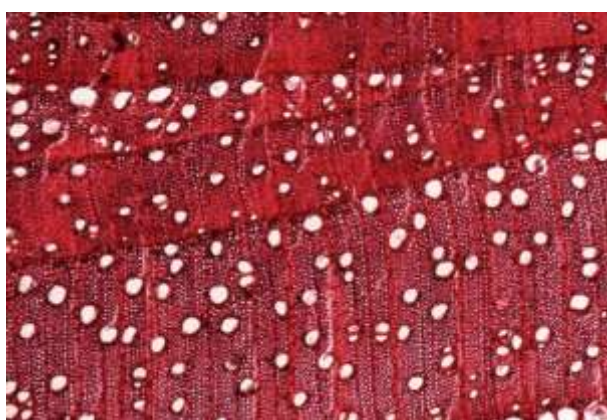
Figure 7. Cross section showing almost exclusively solitary pores with confluent parenchyma (40x).
