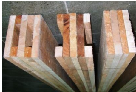
Figure 1. The three variations of glue-laminated column cross sections
