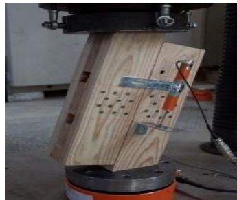
Figure 2. Shear test set up
