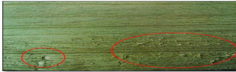
Fig. 4 The planed surface of White Meranti showing torn grain (left), and fuzzy grain (right)
