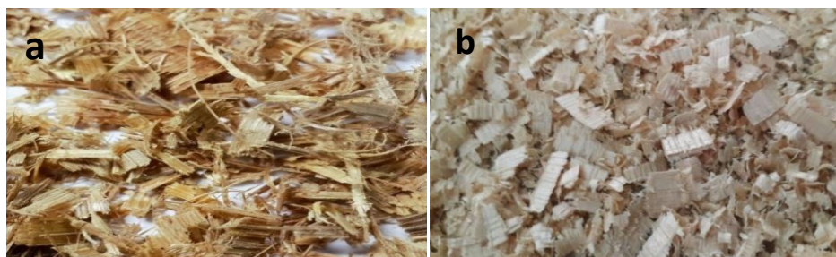
Fig. 6 Comparison of exit particles in the planing of (a) LBT and (b) White Meranti
