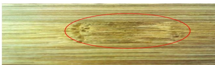
Fig. 3 The planed surface of LBT showing torn grain on the node of bamboo
