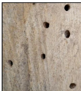
Fig 5. Hole bored and tunnel characteristic (gallery) P. brunnea (Fab.): hole bored at timber K. malaccensis Maing.
