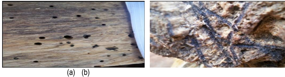
Fig 12. Hole bored P. cylindrus : (a) hole bored and (b) tunnel characteristic at log C. petandra
