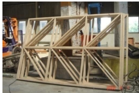
Figure 5. Making the wooden frame LVL shearwall specimens
