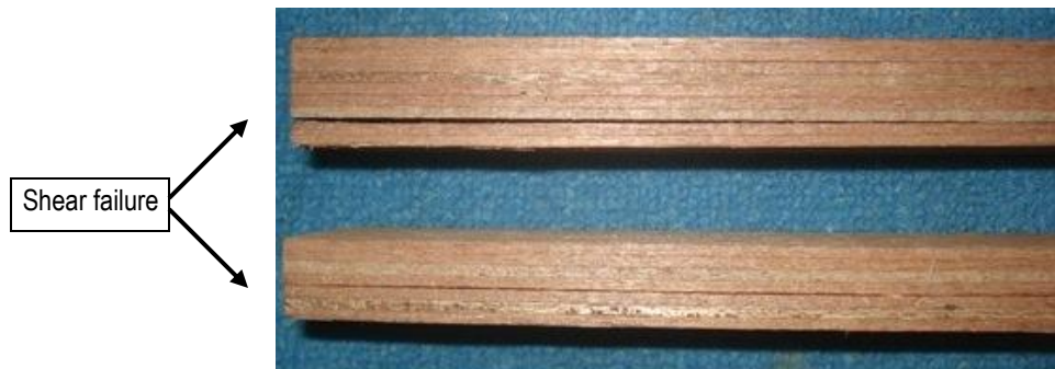
Figure 4. Shear failure after testing
