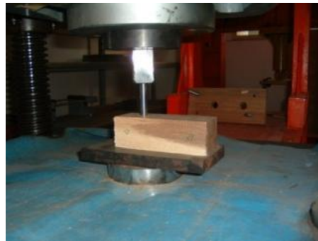
Figure 2. Hardness specimen under perpendicular to the grain test.
