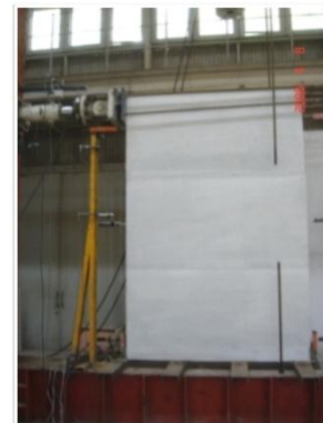
Picture 6. Wood frame shear walls cement board panels
