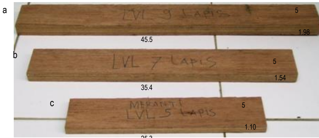
Figure 1. Shape and dimension (cm) of red meranti LVL static bending specimens (a = 9 layer; b = 7 layers; c = 5 layers)
