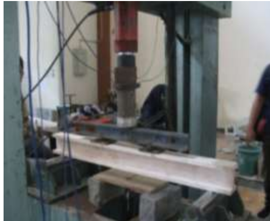
Gambar 4. Setting up pengujian lentur balok LVL kayu sengon
