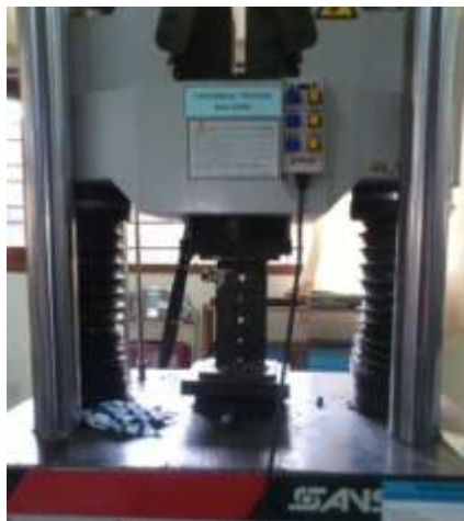
Gambar 3. Setting up pengujian geser paku
